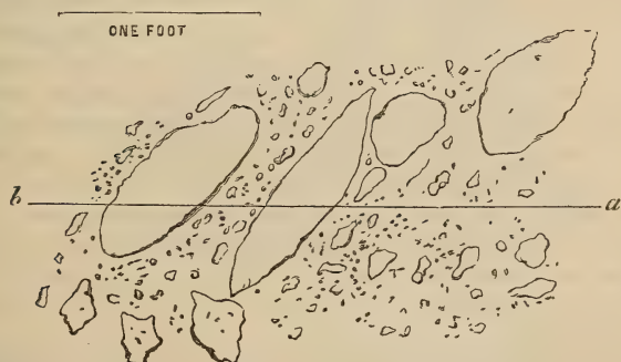
FIG. 219.—PLAN OF COARSE CONGLOMERATE OF BLOCKS OF CAMBRIAN ROCKS IN CARBONIFEROUS LIMESTONE, TRAVERSED BY A LINE JOINT CUTTING THE INDIVIDUAL BOULDERS IN THE LINE a b , COAST NEAR SKERRIES, DUBLIN COUNTY ( B. ).
